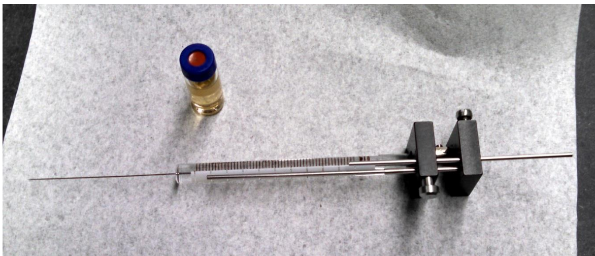
Figure 3: Chaney Adaptor and Vial with Septum Cap
