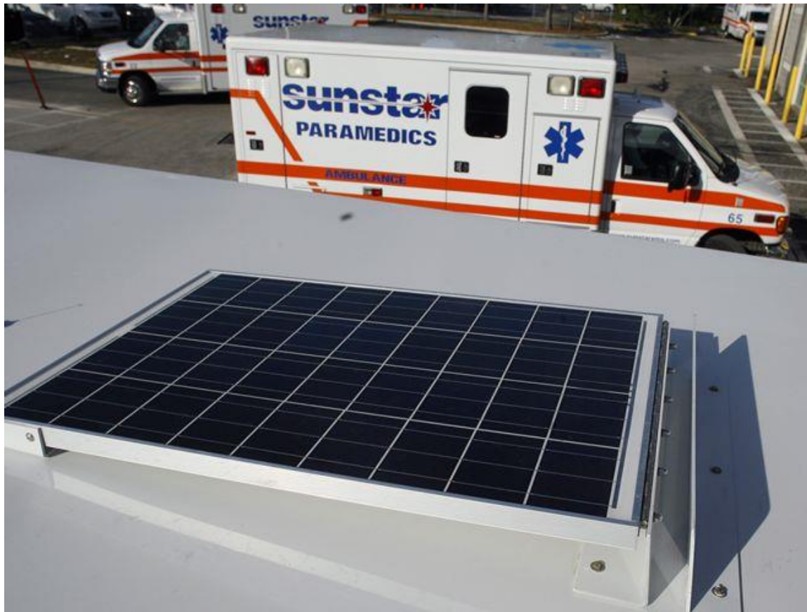
Figure 34 - Solar Power on Ambulance
