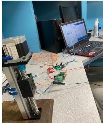
**Figure 5:** Design verification set-up for electrical system. Actuator secured in a ring stand as well as the TB6560 stepper motor driver board, load cell, HX711 load cell amplifier, Arduino board.
