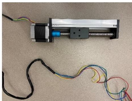
*Figure 2: Ball screw linear stage actuator. NEMA 23 high torque stepper motor positioned at left with colorful wires coming out, stepper motor can spin the screw at the blue cylindrical section, and black rectangular box, “shaft”, displaces along the screw.*
