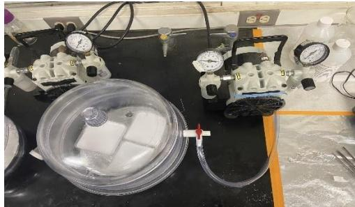
**Figure 12:** Three  $\text{TiO}_2$ -PDMS samples inside vacuum chamber.
