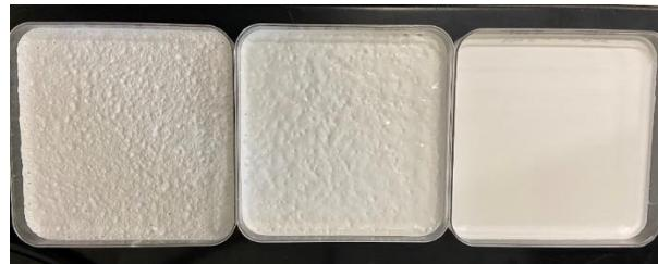
**Figure 14:** 20%, 22.5%, 25%  $\text{TiO}_2$  (vol.) PDMS samples (left to right).
