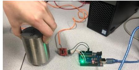
**Figure 6:** Application of an object on top of the load cell. Connections to the HX711 load cell amplifier and subsequently the Arduino board.
