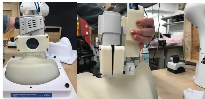
**Figure 18:** Experimental setup for the preliminary testing on a CIRS Thyroid US Training Phantom using Dhirajsinh's pneumatic actuation system as part of the First Experimentation Phase.
