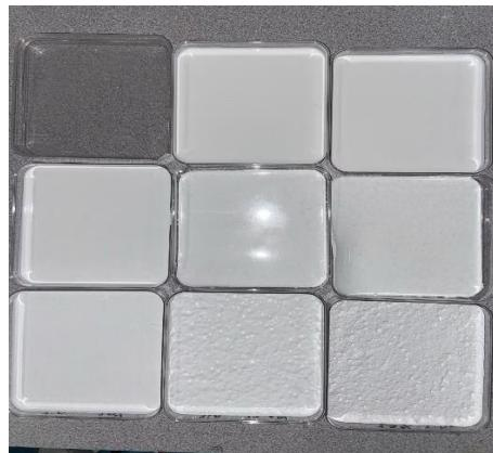
**Figure 15:** 0%, 7.5%, 10.5%,  $\text{TiO}_2$  (vol.) PDMS samples (top left to right); 12.5%, 15%, 17.5%,  $\text{TiO}_2$  (vol.) PDMS samples (middle left to right) and 20%, 22.5%, 25%  $\text{TiO}_2$  (vol.) PDMS samples (bottom left to right).
