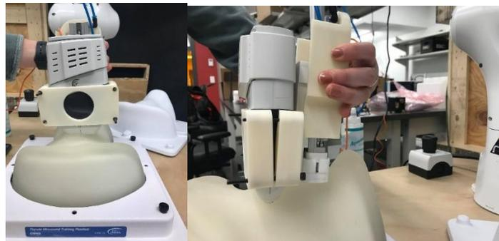
*Figure 18: Experimental setup for the preliminary testing on a CIRS Thyroid US Training Phantom using Dhirajsinh's pneumatic actuation system as part of the First Experimentation Phase.*
