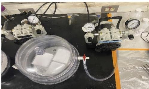
*Figure 12: Three TiO<sub>2</sub>-PDMS samples inside vacuum chamber.*
