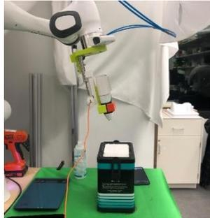
*Figure 20: Experimental set-up for material testing in the Second Experimentation Phase, using a pneumatic system with the Clarius US transducer.*
