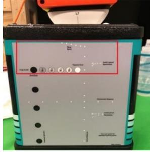
*Figure 17: CIRS General Purpose Phantom with targets of interest outlined in red box.*
