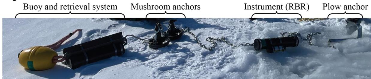
Figure 19. An example of one of the moorings deployed with labelled components. The buoy (yellow) is released on a tether to the surface for retrieval, while the anchors on either side of the instrument secure it to the seafloor. Image courtesy of Jim Thomson.
