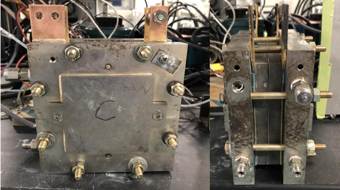
Figure 4.6. Completely assembled cell structure with all internal MEA components enclosed within the graphite bipolar plates in the middle
