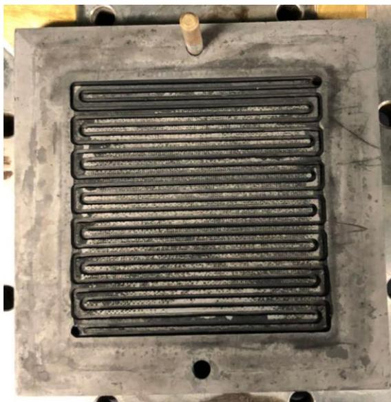
*Figure 5.5. Deteriorated and oxidized graphite bipolar plate*
