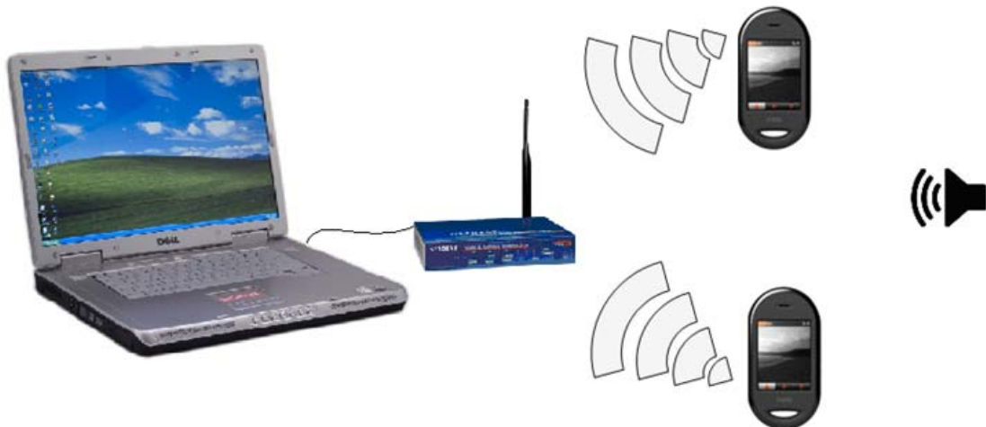
Figure 2 – Illustration of Hardware Setup for Acoustic Localization Using Cell Phones as Sensors and implementing a Central Processing Point. The Two Phones are Used as Sensors to Stream Captured Audio Data Wirelessly Through a Wireless Router to a Central Processing PC (Modified from [Dell Inspiron], [FWG114pv2], and [Openmoko Image, 2009]).
