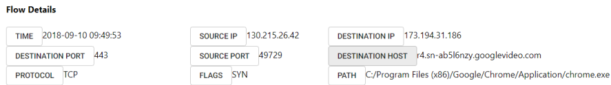
Figure 2: Non-PEACE Flow Elements (General Flow Information) - This element shows the general information a network analyst would have using the current industry standard firewalls
