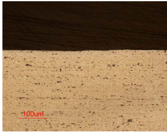
Fig. 4-20 6061-T6 flycut surface after 1100 hrs at 125C, originally imaged at 200X.
