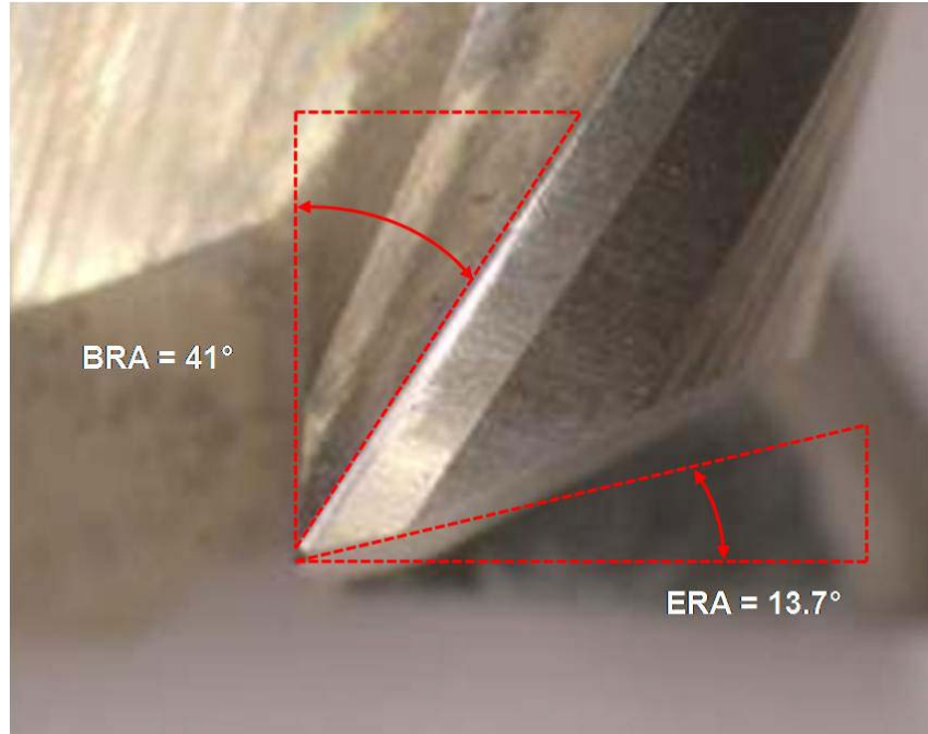
Fig. 4-10 Endmill showing the Back Relief Angle (BRA) and End Relief Angle (ERA).
