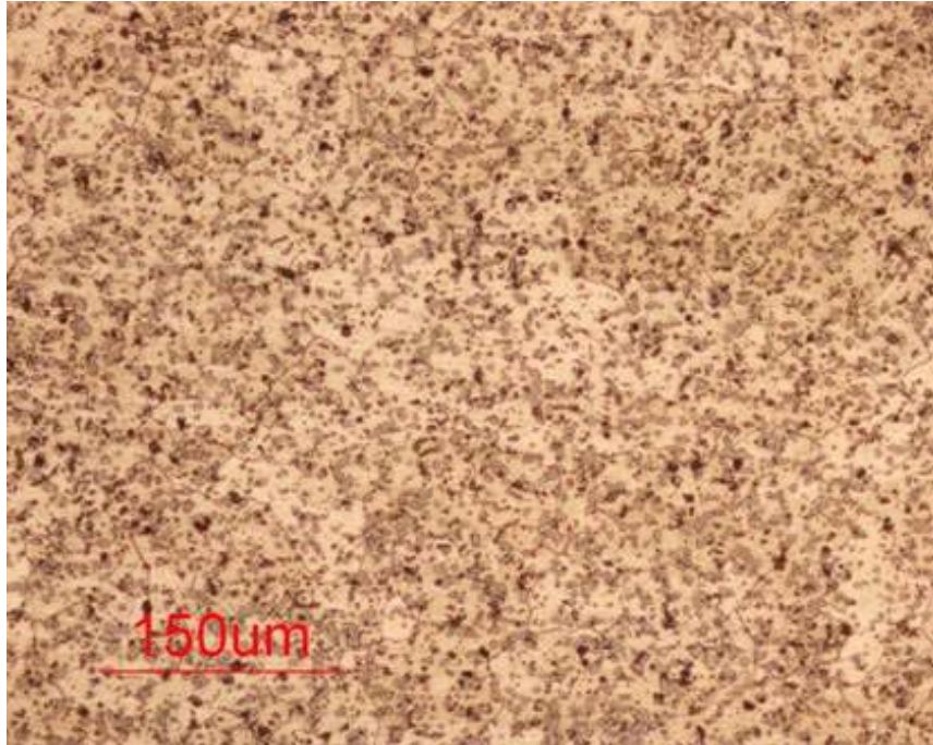
Fig. 4-17 Baseline microstructure of 4032-0 originally imaged at 200X.
