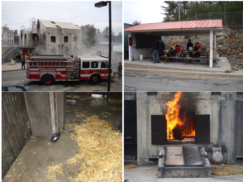
Figure 4.4: Stow Test: MFA Stow Burn Building, Outdoor Reference/Base Station, Indoor Sensor, Flames from Fire Room
