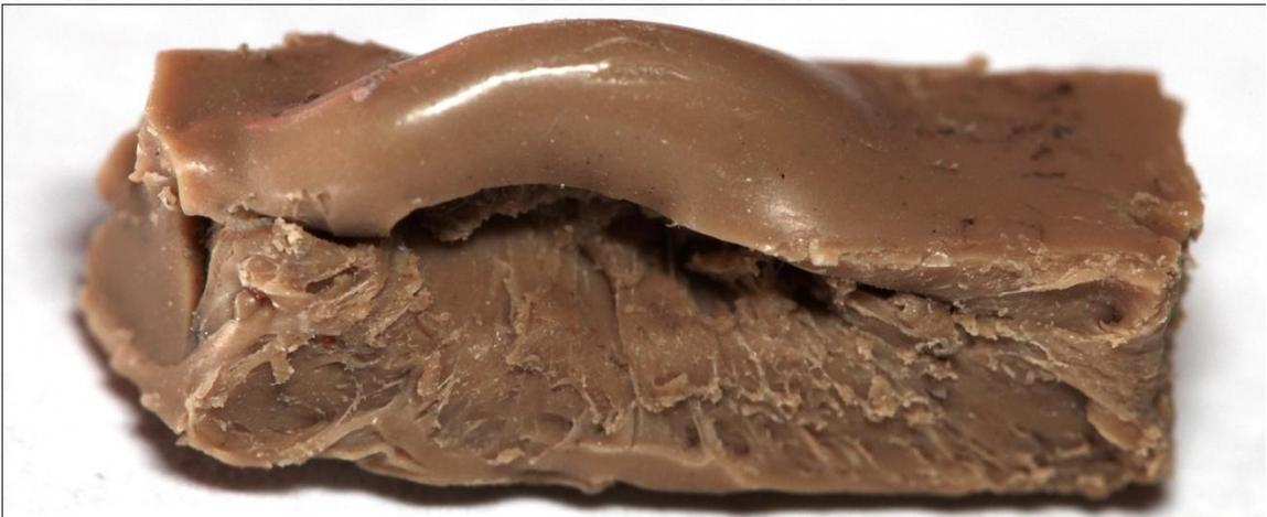
FIGURE 57: NATURAL RUBBER SAMPLE AFTER ONE IMPACT
