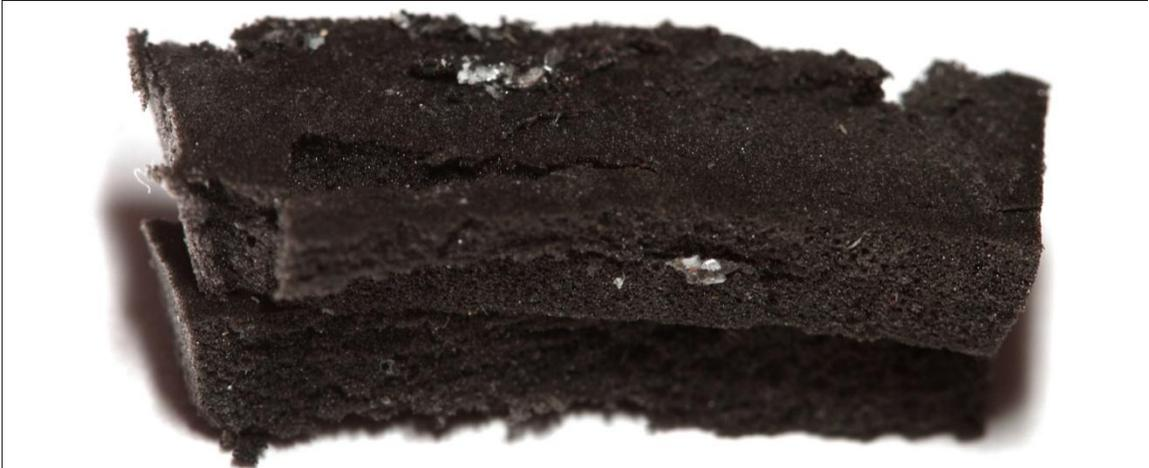
FIGURE 60: POLYURETHANE FOAM RUBBER SAMPLE AFTER ONE IMPACT
