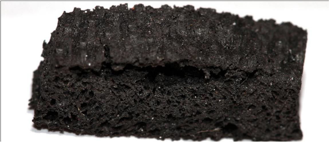
FIGURE 59: NATURAL FOAM GUM RUBBER SAMPLE AFTER ONE IMPACT
