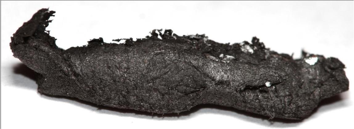
FIGURE 58: EVA FOAM RUBBER SAMPLE AFTER ONE IMPACT
