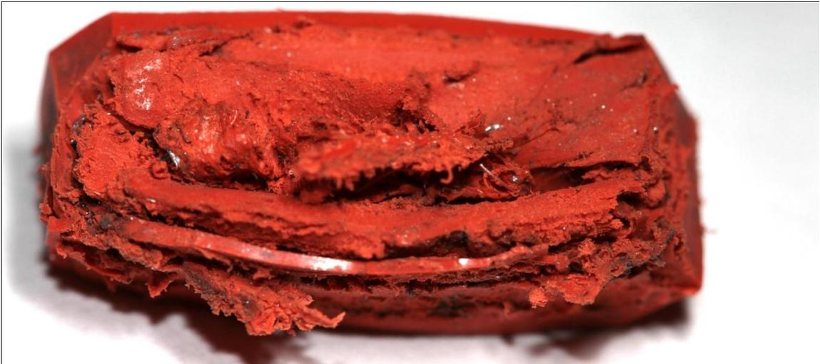
FIGURE 56: 60A SILICON RUBBER SAMPLE AFTER ONE IMPACT
