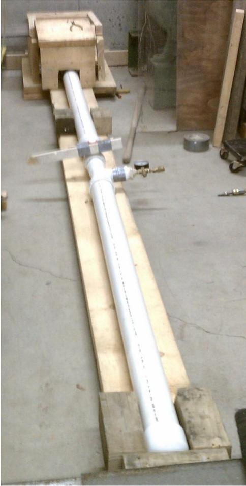
FIGURE 23: RUBBER IMPACT TESTER
