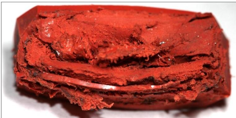
FIGURE 25: 60A SILICON RUBBER SAMPLE AFTER ONE IMPACT
