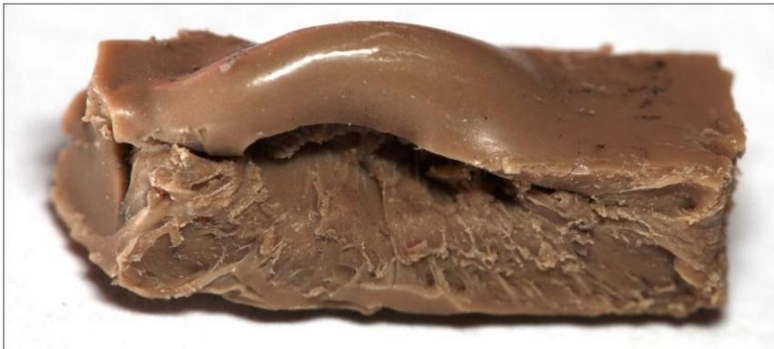
FIGURE 26: NATURAL GUM RUBBER SAMPLE AFTER ONE IMPACT
