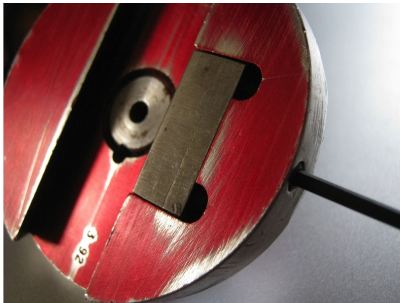
Figure 27: Hex Key on right tightens a set screw that presses the steel plate against the dovetail after it is inserted.
