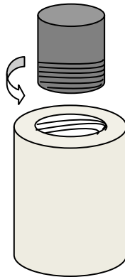
Figure 25: Threaded pipes to align height
