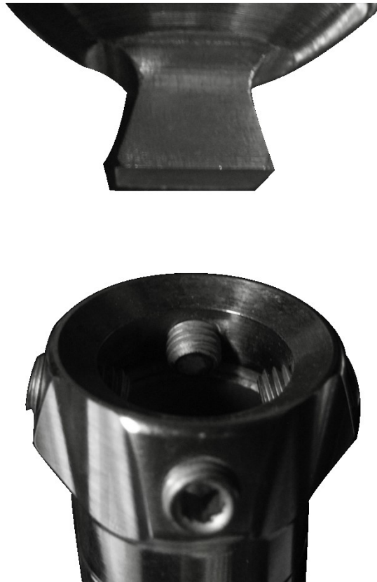
Figure 52: Interface of Module E (Frustopyramid, top) and the tube clamp of the pylon (bottom). The four set screws cause a fixed angle lateromedially and/or anteroposteriorly.
