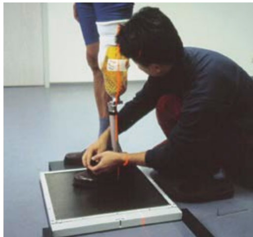
Figure 10: A prosthetist aligning a prosthesis using the LASAR Posture (Otto Bock HealthCare LP)
