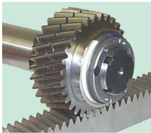
Figure 26: Rack (bottom) and pinion (top) for linear adjustment (JS Auto Tech).
