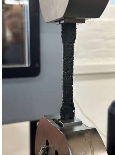
Figure 21: Tensile Test of Dog Bone
