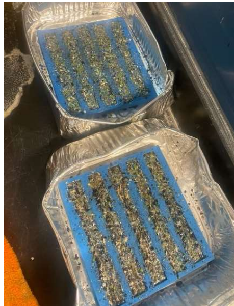
Figure 19: Composite Material Melted into Mold
