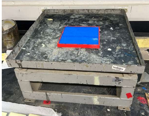
Figure 18: Silicone Mold Formation on Vibrating Table
