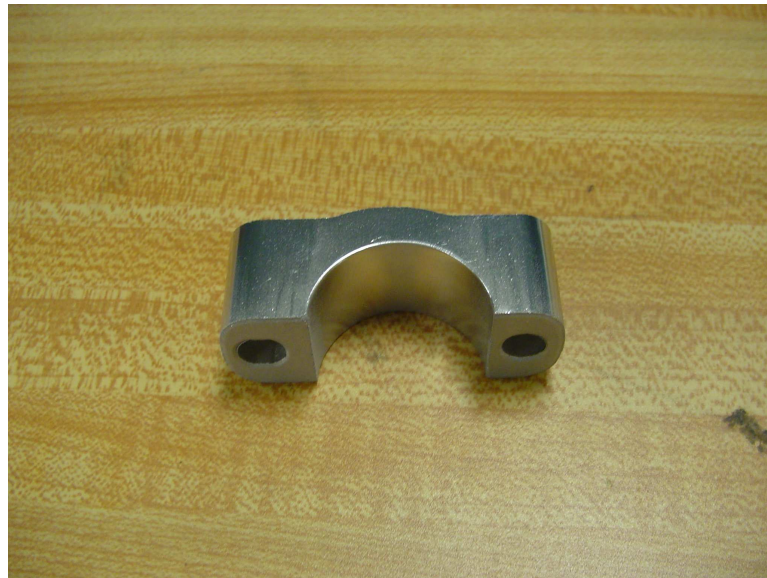
Figure 6.43: Aluminum powder green-state compact (courtesy of MPP Corp., Saint Mary's, PA).
