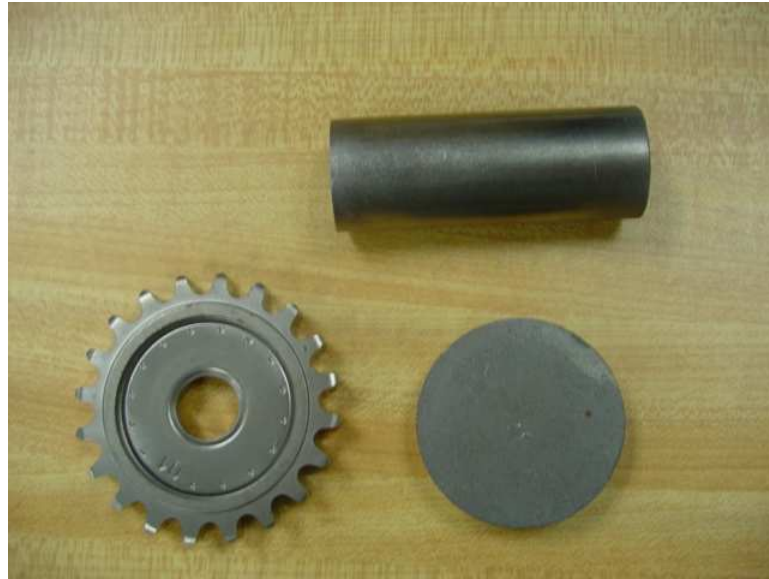
Figure 2.1: Various P/M parts: complex multi-level gear and uniform density cylinders.
