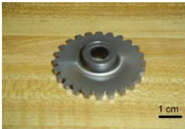
Figure 6.35: Green state P/M compact (part courtesy of MPP Corp., Saint Mary's, PA).
