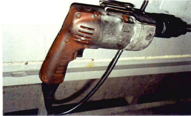
Figure 15: Drill Used to Fasten Screws on RHCo Gate
