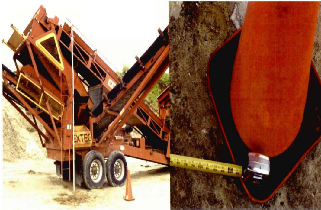
Figure 4: Measurements from Fall Off of Screening Machine's Ladder
