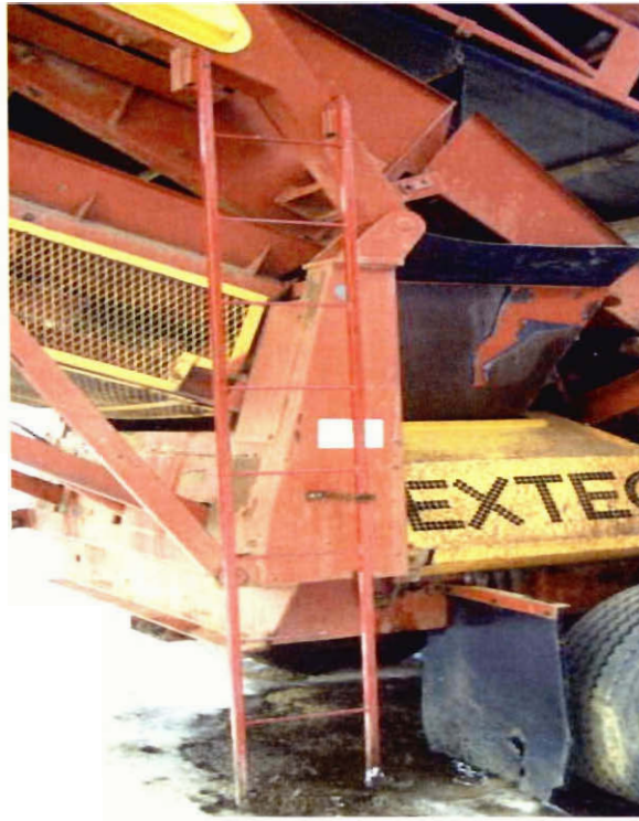
Figure 2: Ladder on Extec Screening Machine
