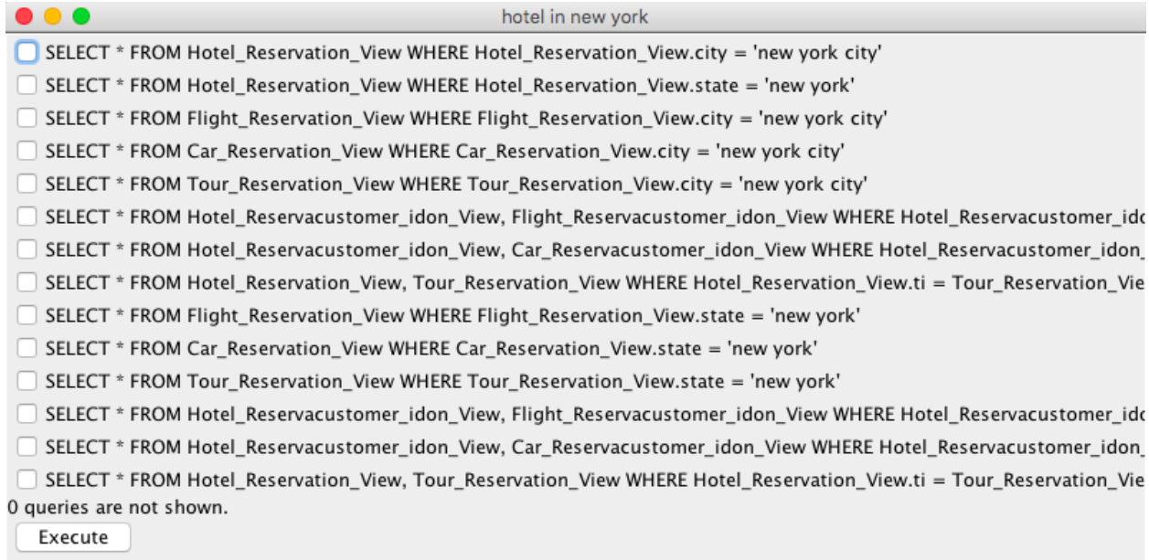
Figure 21: SQL selection screen for “hotel in New York” query. User can select which of the queries that they want to execute. This selection is based on a 0% threshold.
