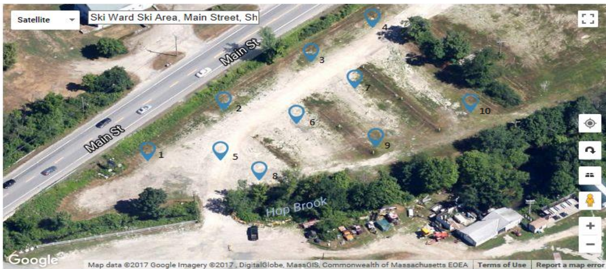
Figure 4.15: This figure shows an aerial view of Lot A along with specific points chosen for elevation data. This figure was key in the design phase when determining the orientation of the French Drain.
