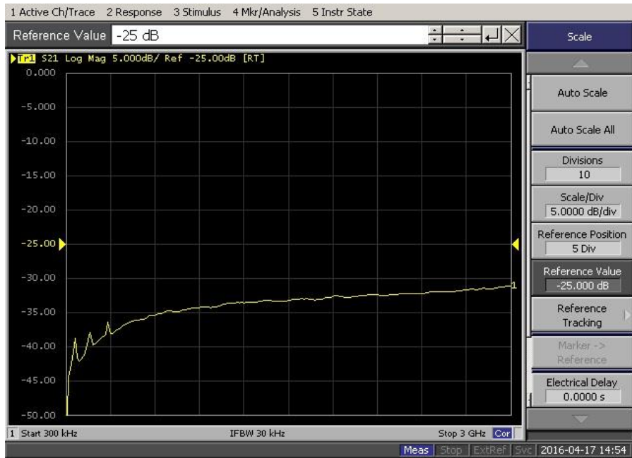
Figure 5.4. Isolation results of the test switch. Frequency was swept from 300 kHz to 3 GHz.
