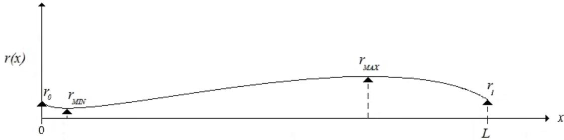
Figure 1 - Cubic Bat Profile from Previous MQP
