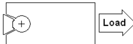
Figure 49 - Shear Tear-out, hole placed too close to edge
