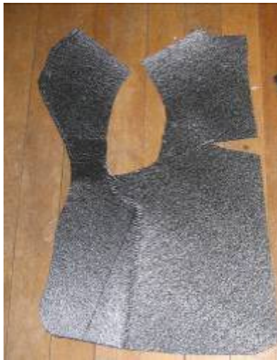
Figure 84 - Ionomer foam pieces sewn together creating a weak construction
