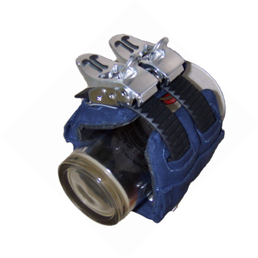
Figure 82 - Final prosthesis attachment strapped to a glass to simulate prosthesis
