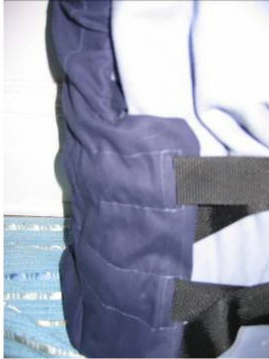
Figure 77 - Close up of the abdominal portion of the vest. Note the nylon straps exiting the sleeves and tailored button holes.
