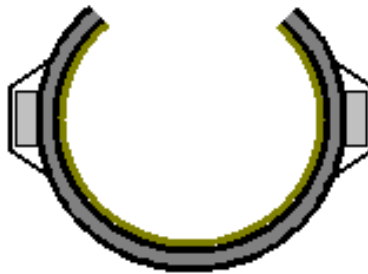
Figure 80 - Cross section of prosthesis attachment showing encased aluminum bars, black is fabric
