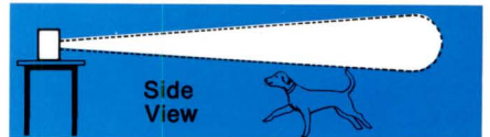
Vertical — 8° plus or minus 15° from the horizontal. The unique aiming lever allows for flexibility in placement of unit so that maximum coverage may be obtained while allowing for movement of pets.
