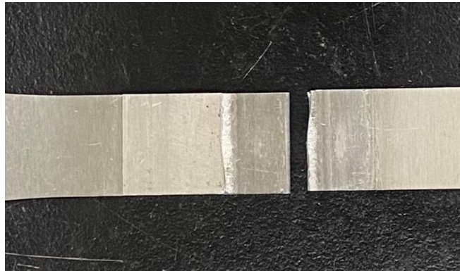
Figure 57 Adhesive-FSW joint failed on ZEK100 Mg after fatigue.
