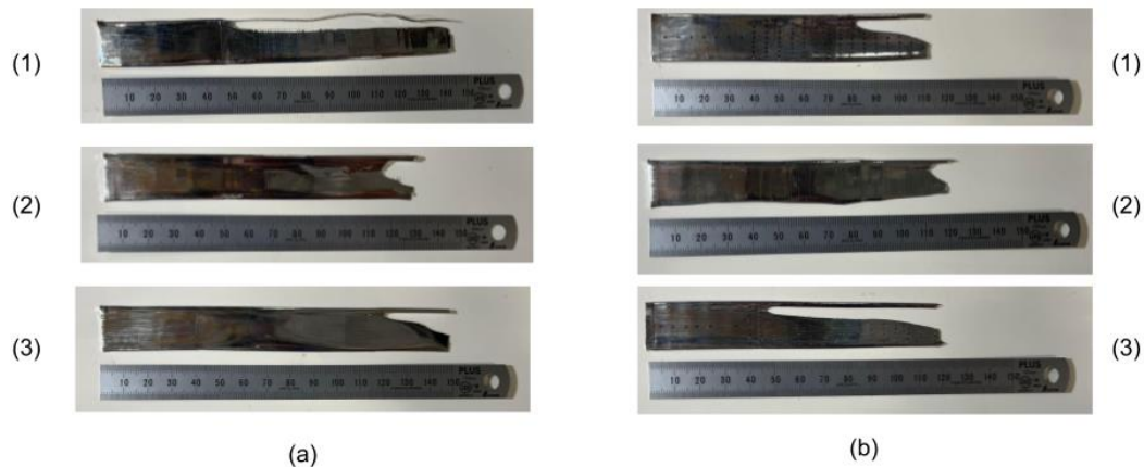
Figure 20: Examples of Successful Alloy U-72 Substrates at (a) 630 kHz and (b) 2.5 MHz
