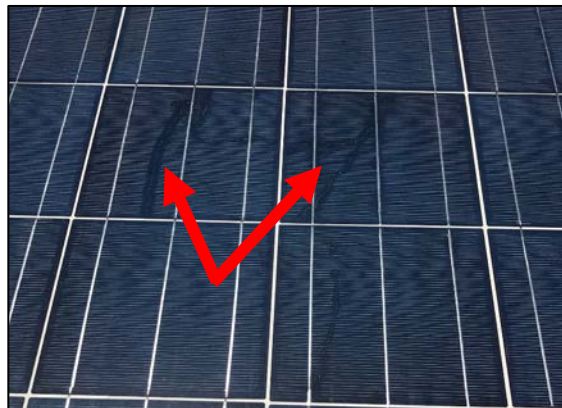
Figure 6: Microfractures that have expanded over time (Fletcher, 2017)
