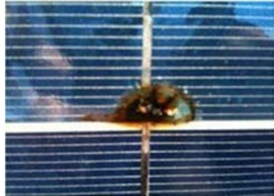
Figure 5: Module Hot Spot Failure (First Green, 2014)
