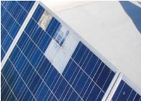
Figure 4: Module Delamination Failure (First Green, 2014)
