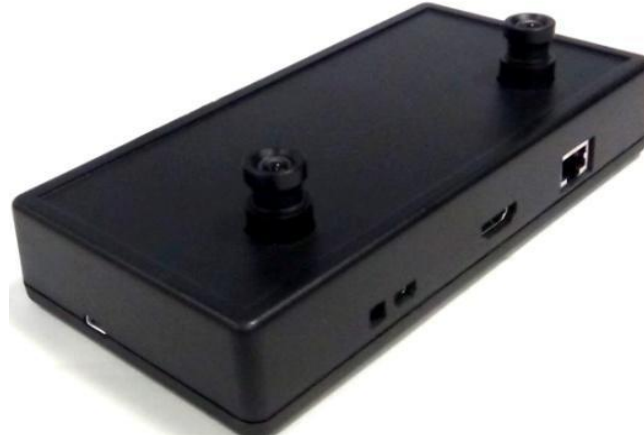
Figure IV.II: Capella Stereo Vision Camera Reference Design
