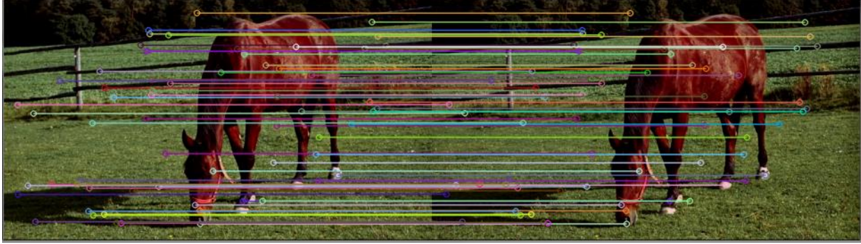
Figure II.VII - Point matching between the images from a stereo camera
