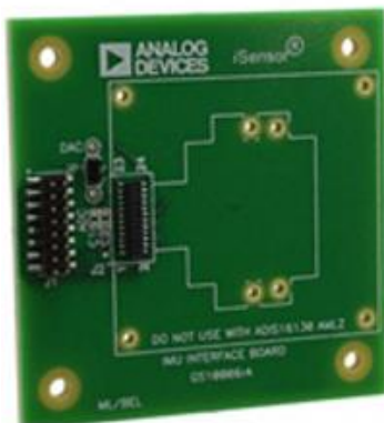
Figure IV.V: ADIS16375 IMU and prototype interface board
