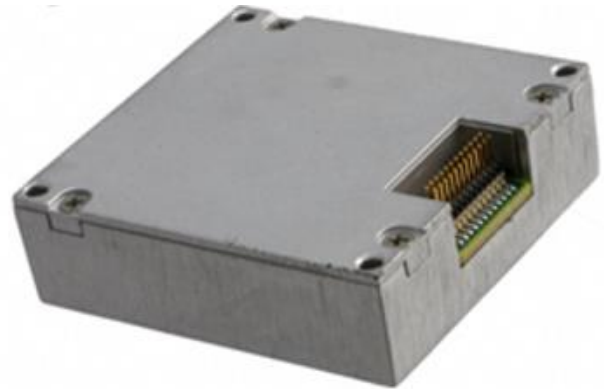
Figure IV.V: ADIS16375 IMU and prototype interface board
