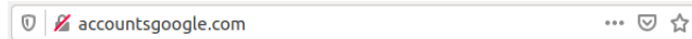
Figure 24: Screenshot of typosquatted domain with HTTP lock warning on participant VM running Mozilla Firefox
