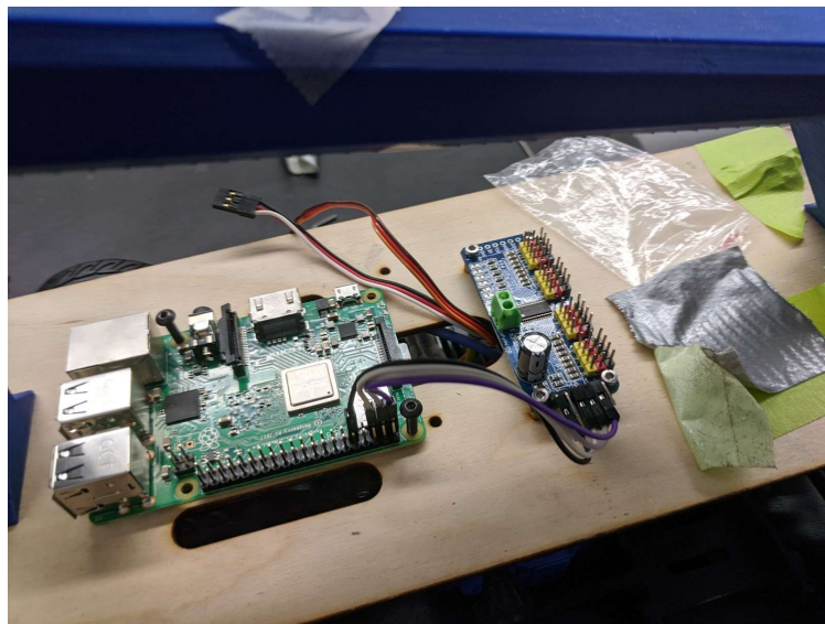
Figure 15. Example of Raspberry Pi and Servo Driver on Car
