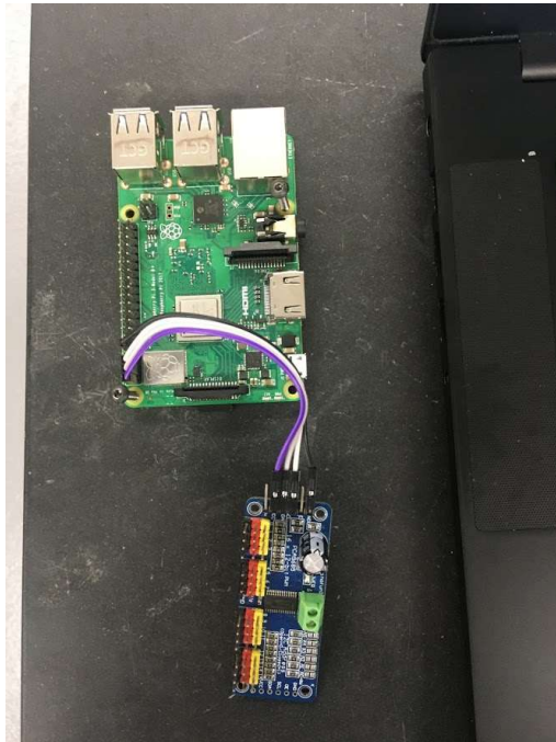
Figure 12. Example of finished Connection between the Raspberry Pi and the Servo Driver
