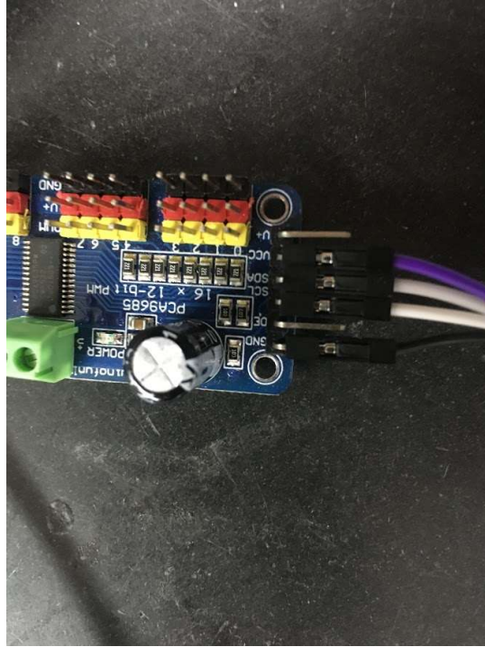
Figure 13. 2nd Example of the connection between the Raspberry Pi and the Servo Driver
