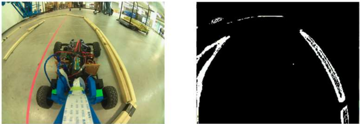
Figure 2.1: Image Masking Example. This particular masking function is meant to highlight the borders of the track to help the Neural Network find a pattern in the data.
