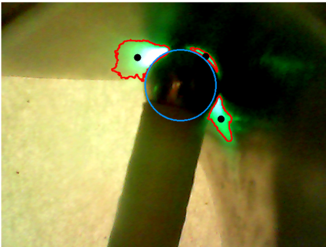
Fig. 41: Identifying the ball gauge location, shown as the bright green circle.
