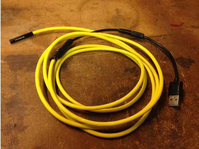
Fig. 32: The GiraffeCam 1.0, a flexible endoscopic camera.
