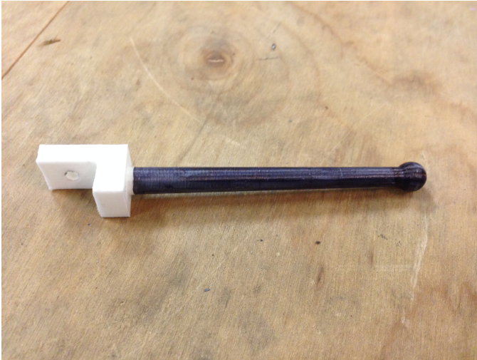
Fig. 29: One of the ball gauges 3D printed for this project. Black Sharpie was used to reduce the light diffusing through the plastic.
