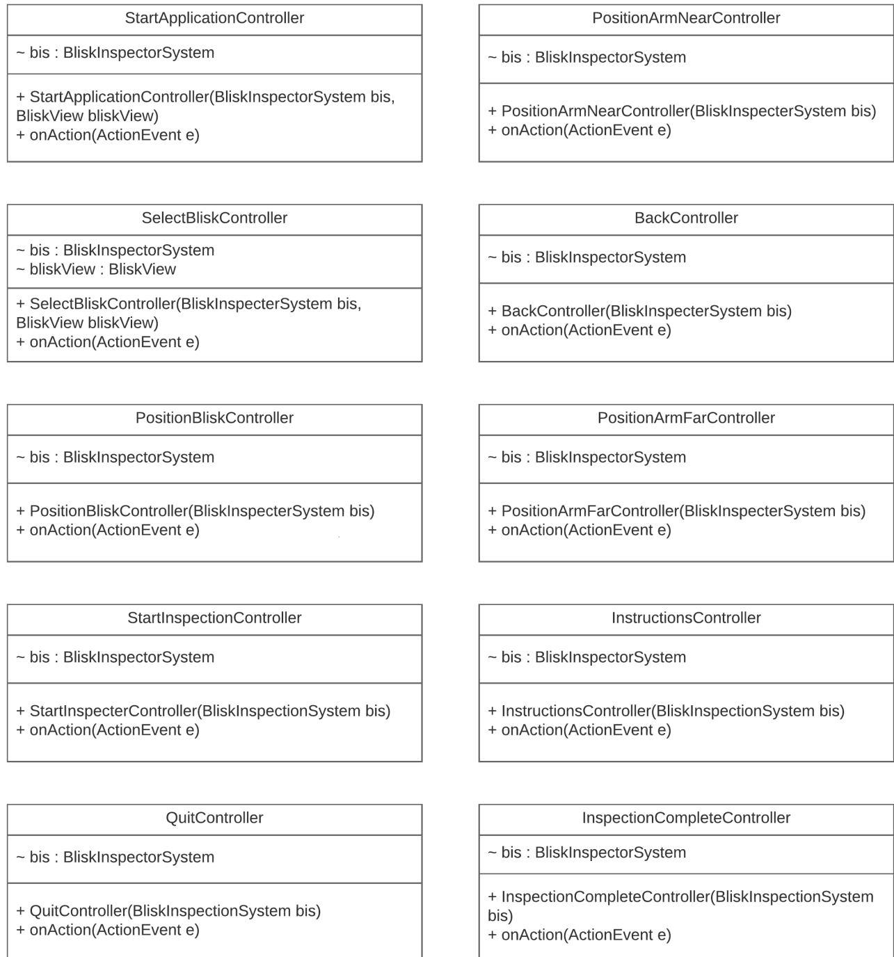
Fig. 48: Controller Class Diagram
