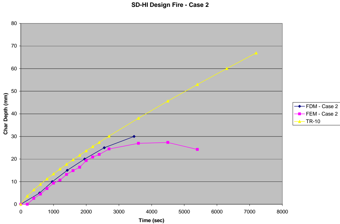
Figure 43 - FDM vs. FEM Case 2 - SD-HI Compared to TR-10 Char Depth for ASTM E-119 Exposure
