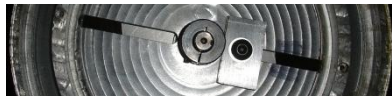
Figure 23. 82g unbalance mass at radius \approx 27mm. It can be moved to radius of 72mm.
