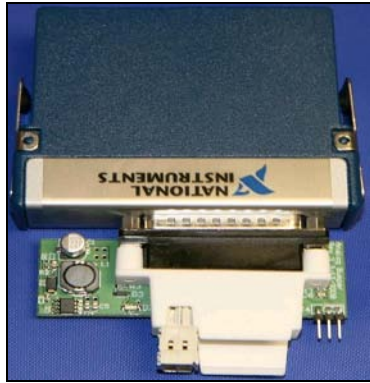
Figure-1: Analog Input Module and Bumper http://first.wpi.edu/FRC/analog.html
