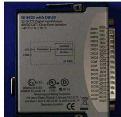
Figure-2: Digital I/O Module http://first.wpi.edu/FRC/digital.html
