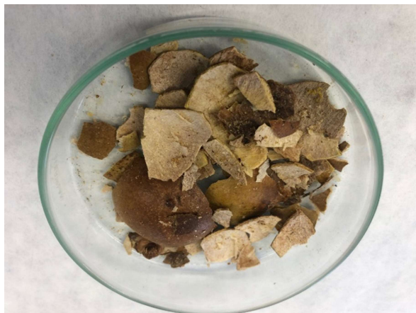
Figure 3.2: Macauba Shells from biodiesel production plant
