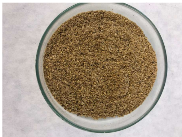
Figure 3.3: Physically Pretreated Macauba Shells
