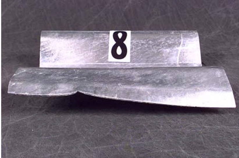
Figure 86: Typical backup plate damage.(17)
