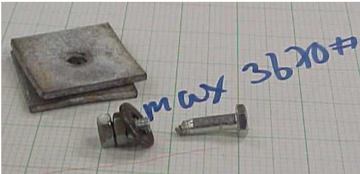
Figure 45: Result of test 99101102 shows the failed components.
