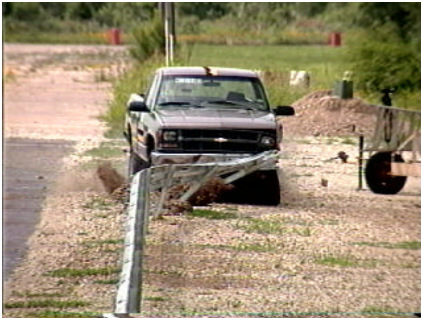
Figure 99: Crash sequence at time » 0.30 sec (TTI 473750-3).
