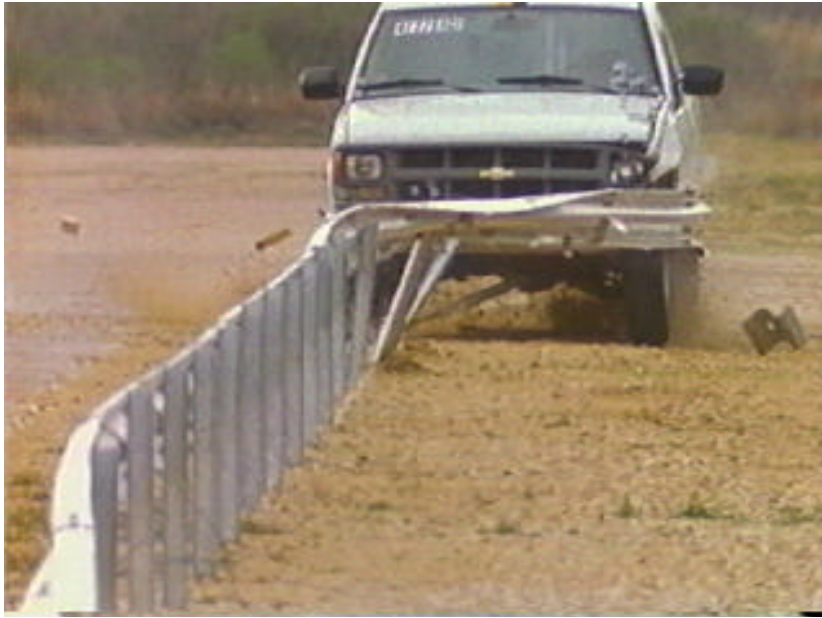
Figure 81: Crash sequence at time » 0.3 sec (TTI 473750-2).
