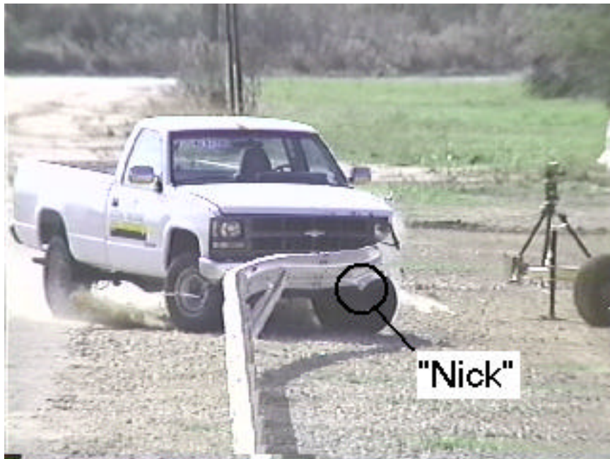
Figure 50: Crash sequence just before rail rupture (TTI 473750-1).
