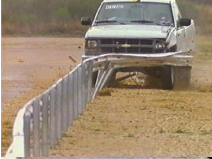
Figure 82: Crash sequence at time » 0.4 sec (TTI 473750-2).
