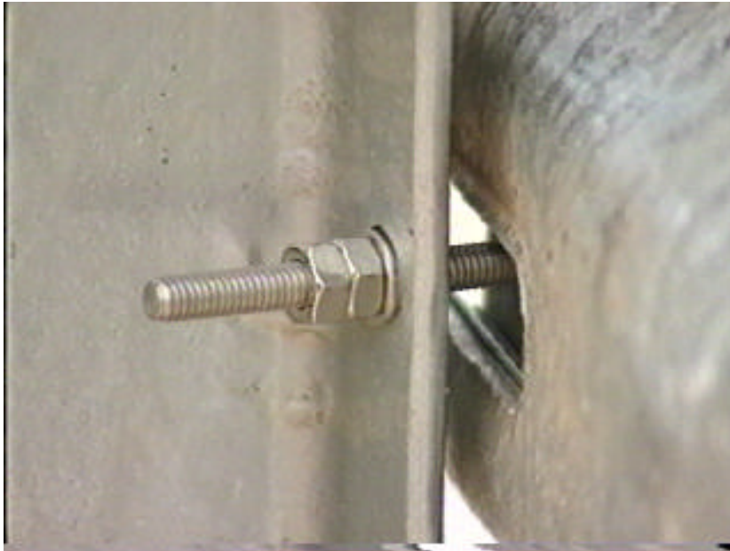
Figure 78: Guardrail and backup plate mounted on a 6-mm diameter bolt with increased length.
