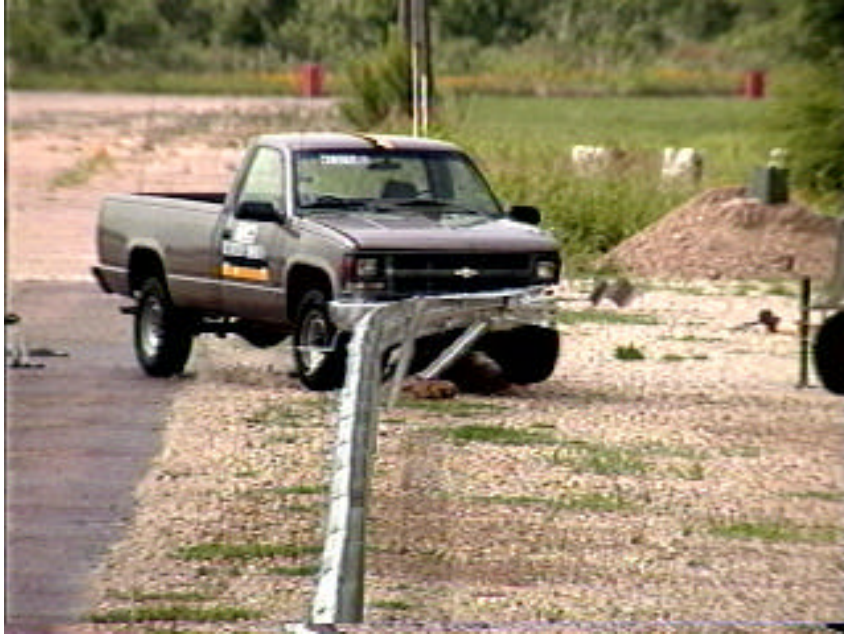
Figure 98: Crash sequence at time » 0.18 sec (TTI 473750-3).
