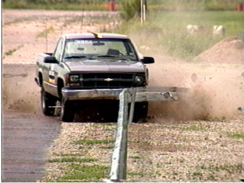
Figure 102: Crash sequence at time » 1.20 sec (TTI 473750-3).
