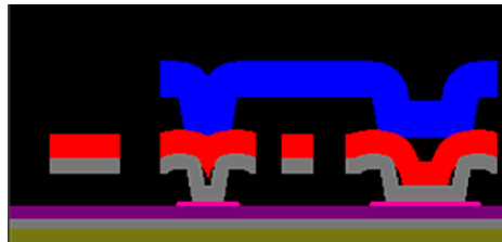
Fig. 2.6. 2D representation of the cross section of the anchor hinge along line A-A (Pryputniewicz and Furlong, 2003).
