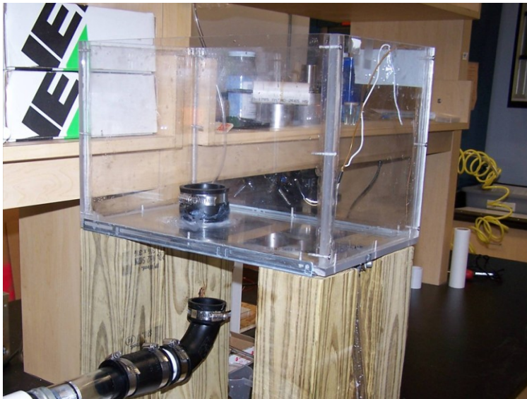
Figure 4.6 Clear plastic tank for submersion of models
