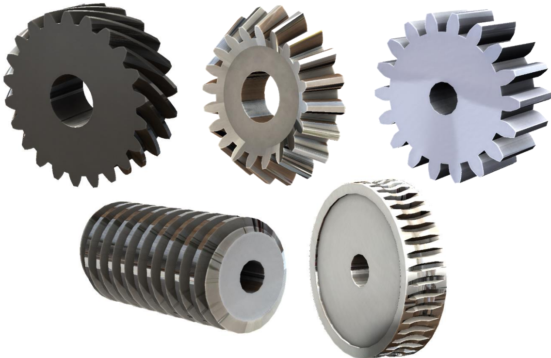
Figure 13. SolidWorks Gears Generated by the tool. (Helical, Bevel, spur, Worm, Worm wheel)
