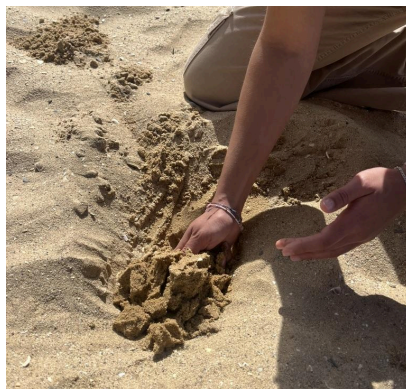
Figure 14. Illustrates sand collection at Playa de Getares. Topsoil must be collected (7-10 centimeters deep) to ensure accurate test results.
