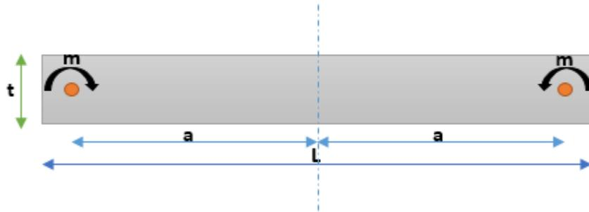
Figure 34: FBD of Beam in Pure Bending
