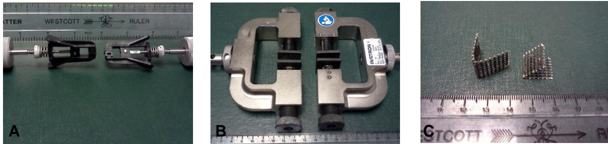
Figure 51: Mechanical Testing Setup Accessories. Figure A is the small grips that were first used; Figure B is the large grips; and Figure C is the sandpaper meshes.
