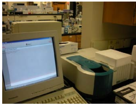
Figure 10 - Cary UV Spectrophotometer
