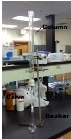
Figure 11 – Column Adsorption Test
