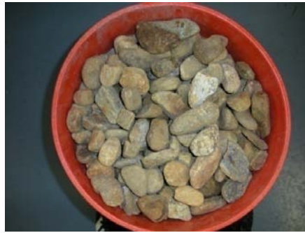
Figure 14 - Recharge Bed Aggregate
