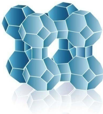
Figure 8 - Tetrahedral Zeolite Unit Cell (CO2CRC, 2008)
