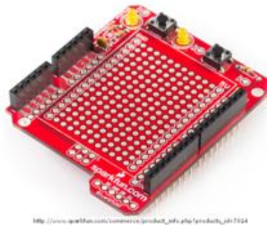
Figure 73: ProtoShield Board (Sparkfun Electronics, 2009).
