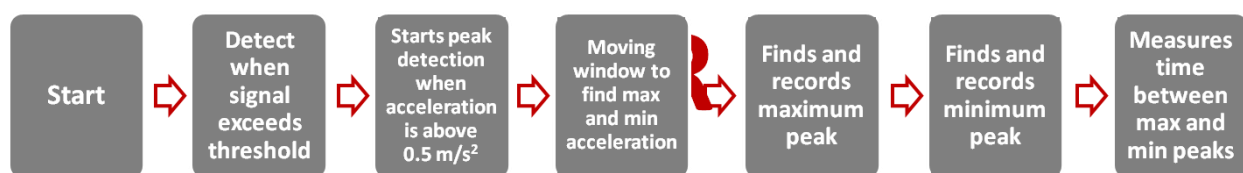
Figure 77: Block Diagram of Final Design.
