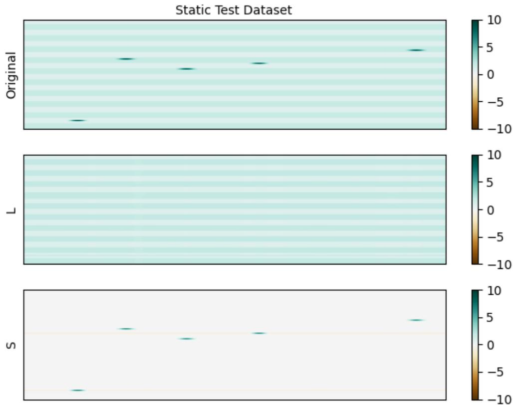
Figure 24: A synthetic example where normal samples are represented by rows with either values of one or values of two. An autoencoder was trained on normal samples only. Anomalous entries contain features with a value of five. One can see that after training on normal samples,  $L^k$  is dominated by values of all ones or all twos, while  $S^k$  is sparse and contains the anomalies.
