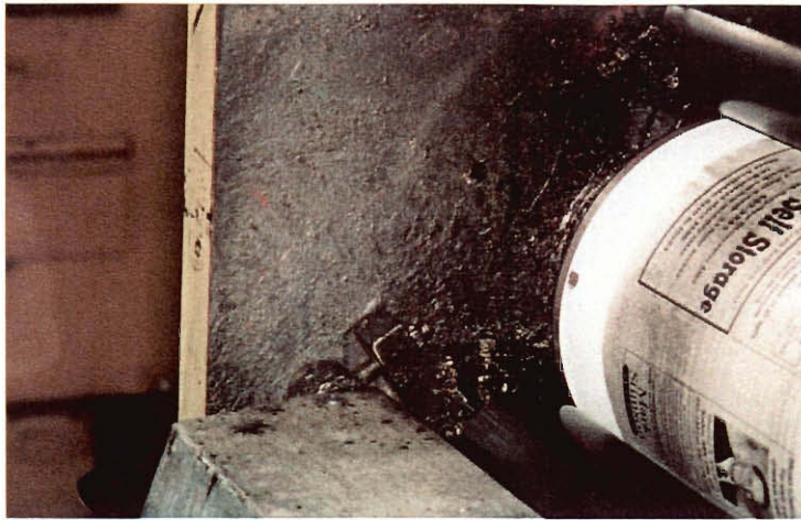
Figure 12: A 'hickey' on the End of the Roller
