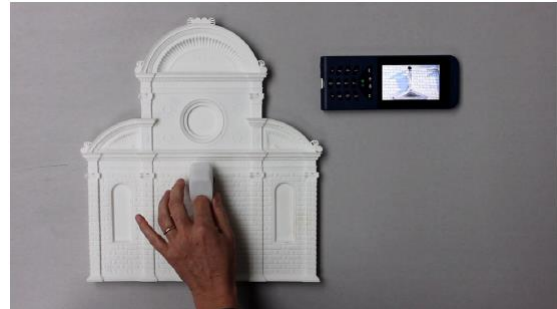
Figure 9: Facade with RFID Tag and device
