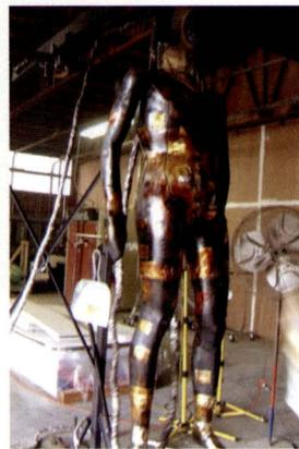
Burns to the lower extremities, visible on a tested firefighter's suit (above), register as torso burns via copper slug skin calorimeters on the mannequin (left). The suit is made from polybenzimidazole (PBI), a material used in most firefighters' suits. "Part of the reason for the extent of these burns," says Jay Kramarczyk '04, lab assistant in WPI's burn chamber, "is that the scenario the suit is exposed
