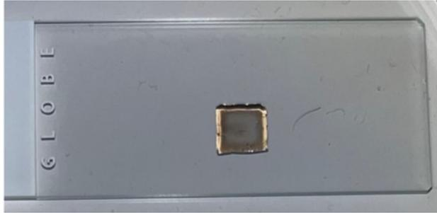
Figure 1.11: SF film on a microscope slide.
