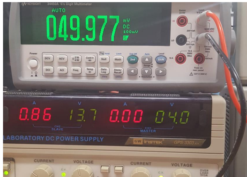
Figure 6.12: Voltage Across MOSFET, Gate Voltage Equal to 4.0
