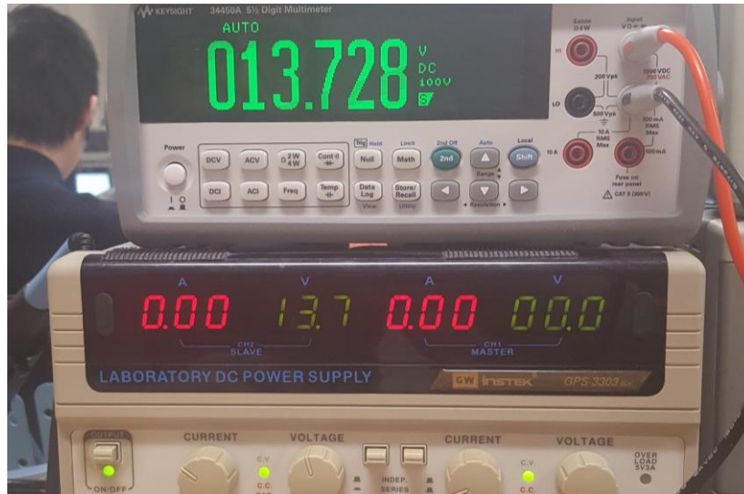
Figure 6.13: Voltage Across Load Resistors, Gate Voltage Equal to 4V
