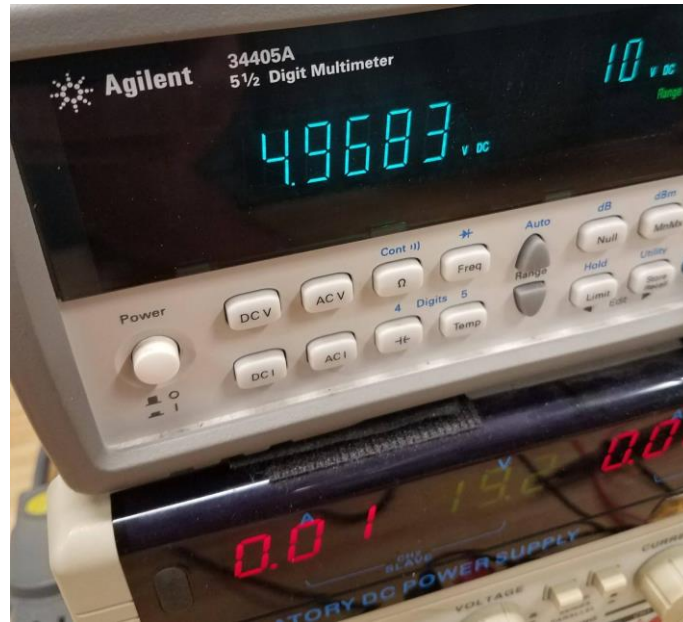
Figure 5.5: 5 Volts Out with 19.2 Volts In, Variable Current
