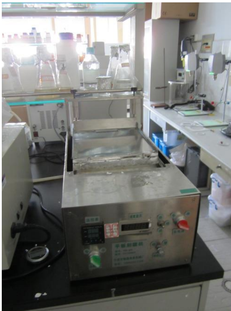
Figure 19: This machine evenly distributes the casting solutions across the glass plates at a specified thickness
