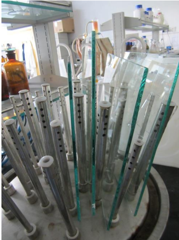
Figure 18: The glass plates that the casting solutions are poured onto
