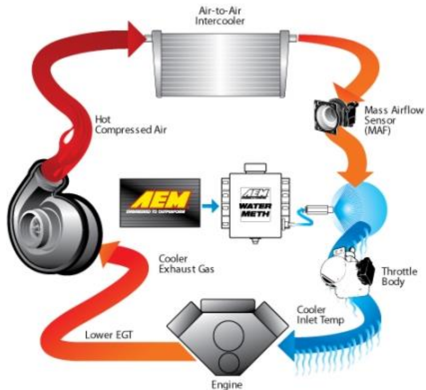
Figure 43: Methanol Injection Kit Diagram [66]
