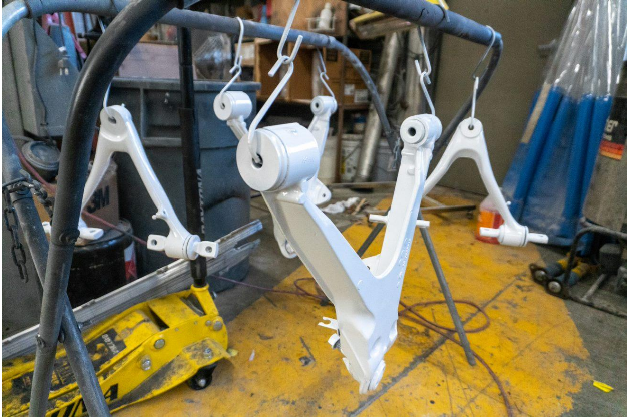
Figure 48: Bushings Installed into Control Arm
