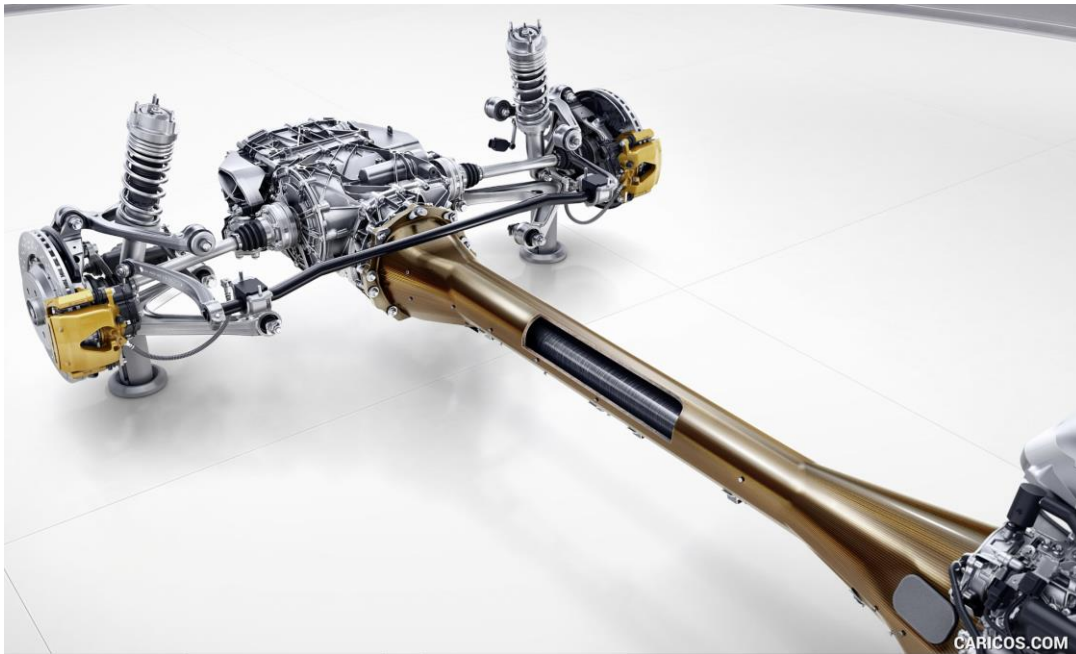
Figure 17: Torque Tube Connecting Engine and Rear Transaxle [26]
