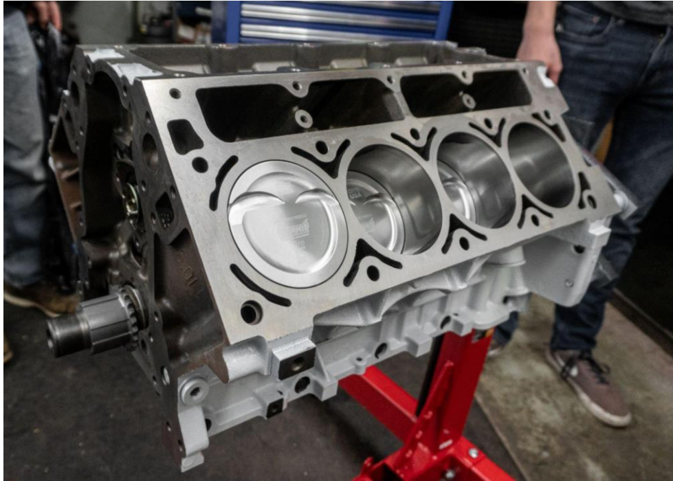
Figure 36: Engine Block after Installation of Crank, Camshaft, Piston, and Rod Assemblies
