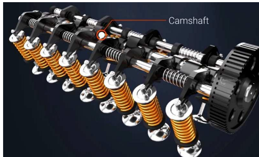
Figure 14: Diagram and Image Depicting Overhead Style Orientation [18]
