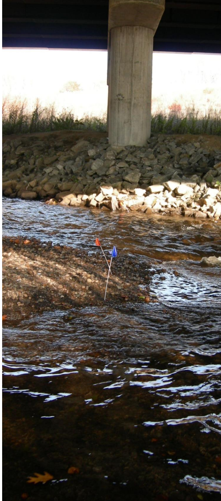
Figure 15: Transsections 2 and 3 (view from far bank of 3 to near bank of 2). Note that all test points for both transsections are in line with the three columns
